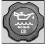
The engine oil fill cap is located on the passenger's side valve cover. See "Engine Compartment Overview" in the Index for more information on location.
